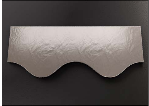
Figure 48: Fabricating the insulation for valve connection
