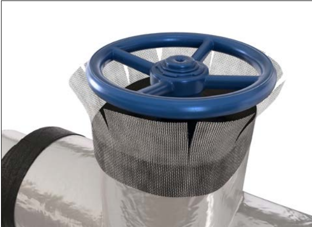
Figure 56: Application of the flexible reinforcement membrane at spindle insulation termination
