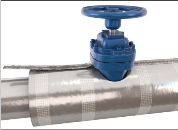
Figure 42: Application of vapour barrier tape
