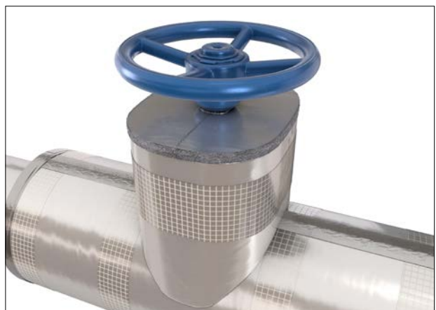
Figure 50: Insulate the top of valve spindle
