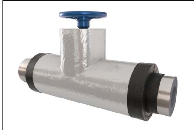
Figure 53: Application of vapour stop
