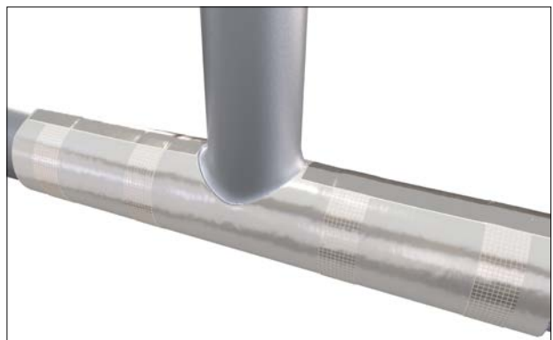
Figure 24: Securing equal tee with vapour barrier tape
