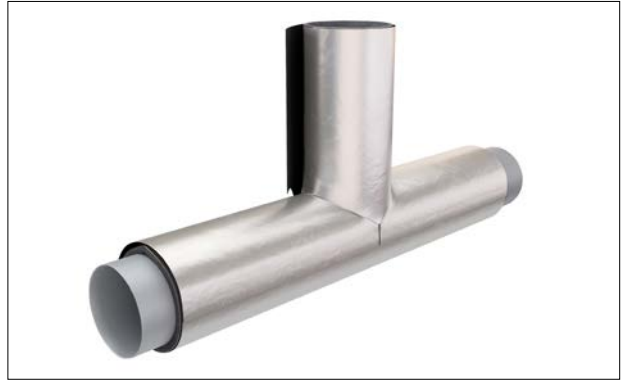
Figure 75: Application of primary vapour barrier on tee
