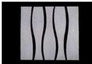
Figure 34: Cut gores to suit exact circumference of pipe. Remember to allow a half starter / finisher piece.
