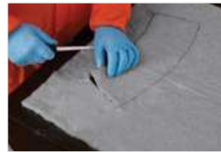
Figure 43: Cut radiused strip.
