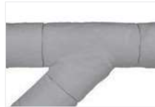
Figure 53: Install oblique angled branch and wire into place ensuring that all joints are tight without gaps.
