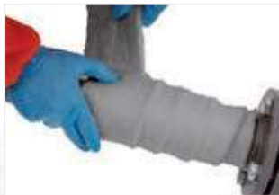
Figure 28: Wrap 50 or 100 mm wide strips of ArmaGel HT around pipe. Material can either be close butted or overlapped by 50%.
