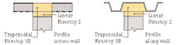
Figure 1 Profiled metal deck over blockwork wall
