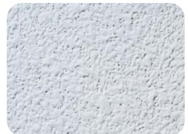
Rockfon stone wool - resin bonded mineral wool tile showing no micro-organism growth
